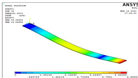
**Fig. 2. Second Mode Shape of Fixed Free Aluminium Beam.**
