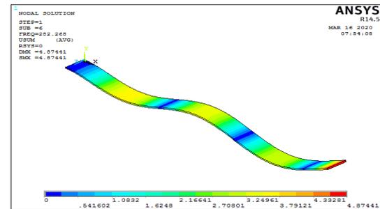
**Fig. 4. Fourth Mode Shape of Fixed Free Aluminium Beam.**
