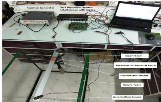
Fig. 6. Experimental Setup.
