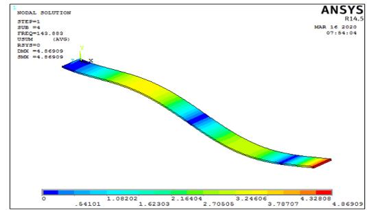
**Fig. 3. Third Mode Shape of Fixed Free Aluminium Beam.**
