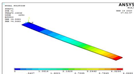
**Fig. 1. First Mode Shape of Fixed Free Aluminium Beam.**
